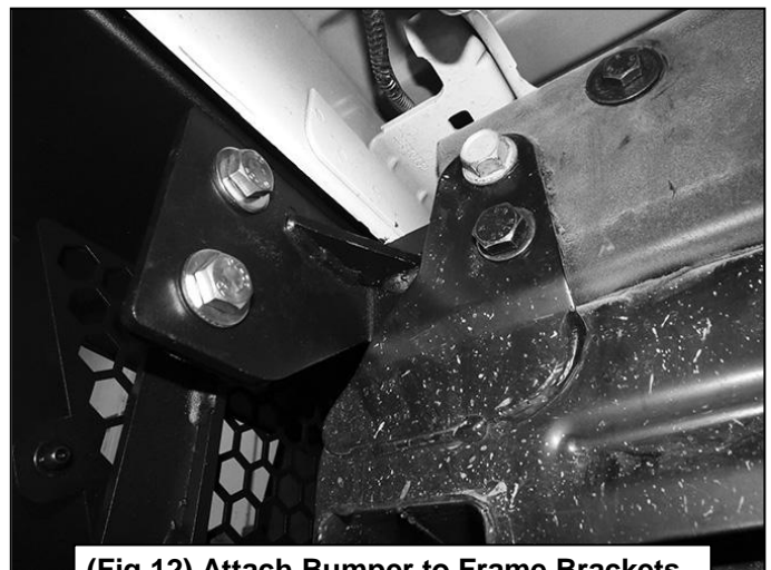
(Fig 12) Attach Bumper to Frame Brackets
